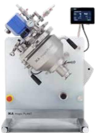
The IKА magic PLANT is an ideal laboratory scale process plant. This system is used for batch-wise mixing, homogenizing, emulsifying, in addition to forming sample suspensions for capacities of up to 2 liters. Whether it is involved with the manufacturing of liquids, pastes or powders – the magic PLANT delivers, enabling a seamless transition from product development to production.
